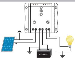
Be aware that the positive terminals of the SMC controller are connected internally and therefore have the same electrical potential. if any grounding is required , always do this on the positive wires.
