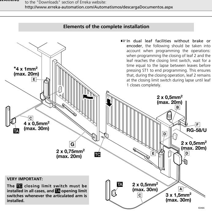
■ The electrolock is obligatory for operators without lock (CL210 and CL250). For operators with lock, the electrolock must be used for gate leaf lengths of over 1.8m.
