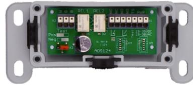
The AOS 124 was developed as a general-purpose control unit for optoelectronic safety edges. The AOS 124 can easily be integrated into the control system as a safety device.
